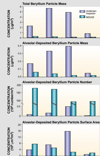
Figure 2. Concentration of the mass, number, and surface area of alveolar-deposited beryllium particles from Andersen impactor and MOUDI samples collected in different process areas
